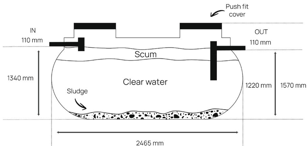
Cross section diagram of Nabridas septic tank
